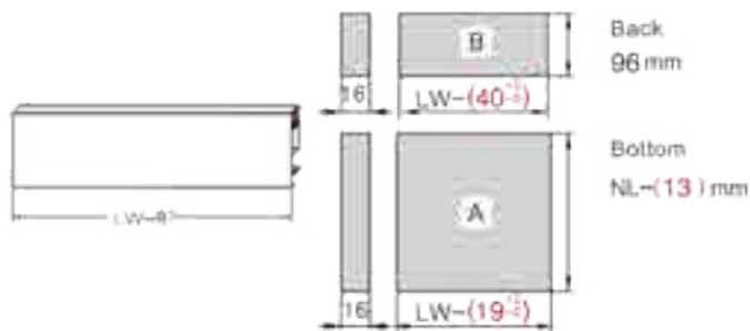
Drawer Front, Back and Bottom Dimensions(mm)
