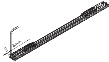
Fix the damper with 3mm allen key
